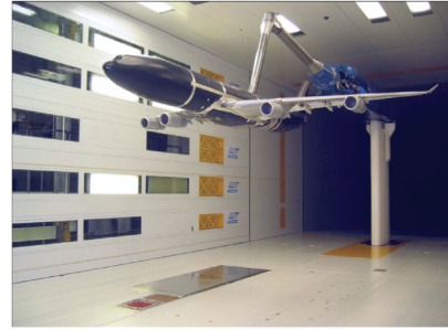
Fig. 28 Test setup in DNW closed test section, with three wall arrays installed on the floor.
